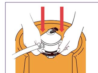
5 With regulator in place, push lock-ring firmly downward until the ball coupling of the regulator is heard to snap into the ball groove or the cylinder valve.
