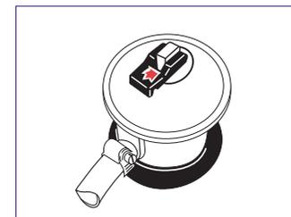
2 Note that in the ON position, the flame symbol on the lever will be visible.
