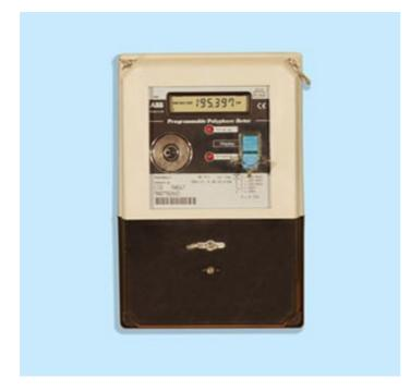
If your RM number is 545 or 667 you may have this meter type. The RM number is at the bottom left hand side of the meter. The meter has an automatic scrolling electronic display. The display changes every 6 secs illustrating 13 different information panels. Flat Rate & Time of Day - use Screens 11, 12 & 13.
