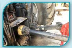
The P.T.O. takes the power from a tractor engine to run a piece of equipment such as a mower or agitator.
