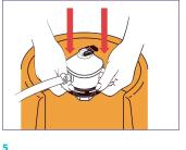
With regulator in place, push lock-ring firmly downward until the ball coupling of the regulator is heard to snap into the ball groove or the cylinder valve.
