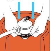
5 Take hold of the regulator at the top and pull upward to check that the regulator is firmly connected to the cylinder valve. If this causes the regulator to become loose from the cylinder valve, the connection was not properly made and must be repeated.
