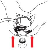
4 With regulator in place, push lock-ring firmly downward until the ball coupling of the regulator is heard to snap into the ball groove or the cylinder valve.
